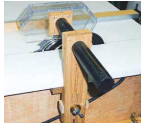
PIC 8. Height adjustment and extraction for the guard
